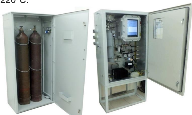
Heated cabinet for MAG GC with cylinder's cabinet
