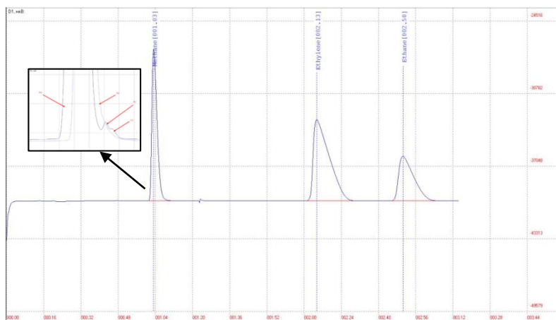
Analytical channel №1 chromatogram (H 2 , CO, CH 4 , ethylene, ethane)
